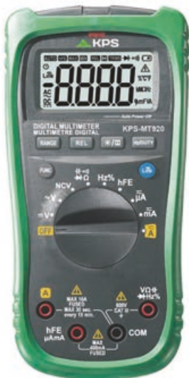
KPS-MT920 TRMS digital multimeter with communication via app
